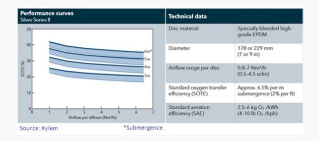
In any case, the SOTE, for practical purposes, will apply the following calculation criterion: For fine bubble diffusers: 6.5% per m diffuser depth.
